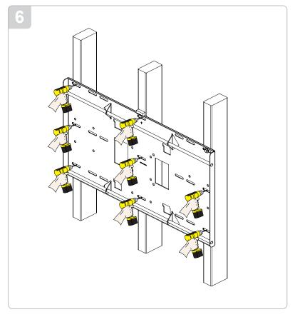
Drill a "pilot hole" in the center of each of the marks with a power drill and a 1/4" drill bit.
