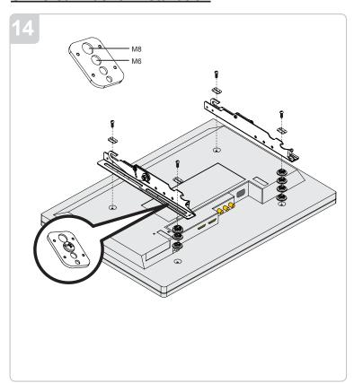
Universal Washers are designed to accommodate the various M6 and M8 hole sizes required by flat-panels.
