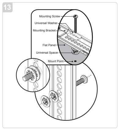
Universal Spacers allow you to attach the mounting bracket to flat-panels which have recessed or uneven mount points. Each Universal Spacer adds 1/4" to the distance between the mounting bracket and your flat-panel.
