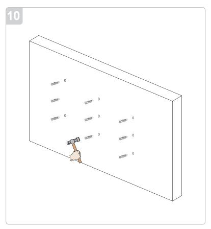
Insert a Finned Anchors into each hole. Lightly tap each Finned Anchors into place with a hammer.
