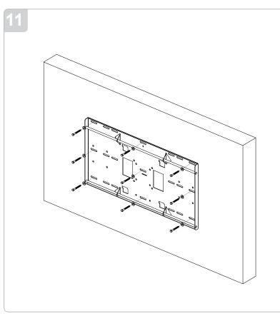
Insert the lag bolts and washers into the Finned Anchors. Tighten all lag bolts using a socket wrench and 1/2" or 13mm socket.
