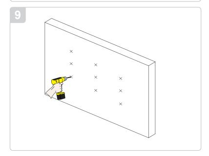
Drill nine (9) pilot holes of each mark using a drill and 3/8" masonary drill bit. Drill 3 inches deep.
