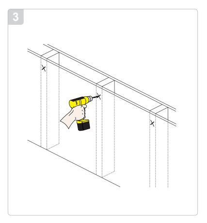
Drill a "pilot hole" in the center of the upper right mark using a 1/4" drill bit and power drill.
